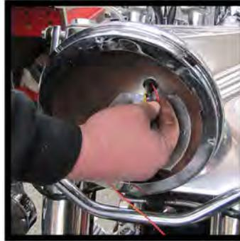
2. Now thread an 18" length of 16-gauge wire through the grommet and out of the left side of the triple tree covers.
