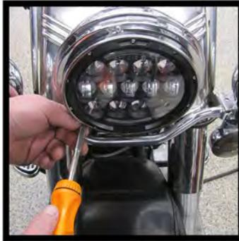
6. Now reinstall the stock beauty ring using the three stock screws and a #2 Phillips screwdriver.
