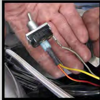
7. Plug the new connector onto the back of the switch. Make sure it is secure. Then reinstall the switch in the left triple tree cover.
