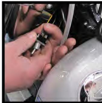
5. Using wire strippers, bare about 3/8" of wire. Also cut the blade connector from the stock wire you just pulled from the spotlight switch with wire cutters and bare about 3/8" of that wire.
