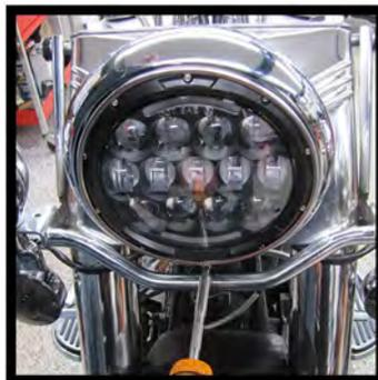
8. The final step is to reinstall the stock trim ring using the stock screw and a #2 Phillips screwdriver.
