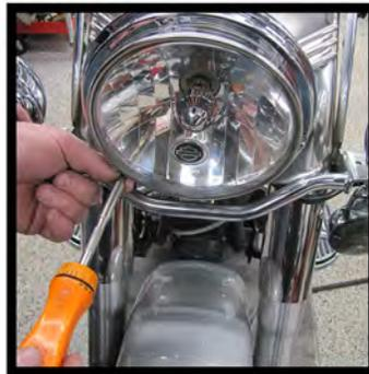
2. Remove the three screws that hold the beauty ring to the headlight bucket using a #2 Phillips screwdriver. Lay this ring and these screws aside for reinstallation later on.
