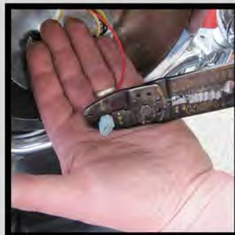
9. Cut the wire you installed so about 7" of it is in the headlight bucket and bare about 3/8" of wire. Then install a female blade connector on the wire and a male connector onto the short red wire on the new LED headlight plug.
